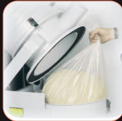
Opening the filter housing for dust bag removal
