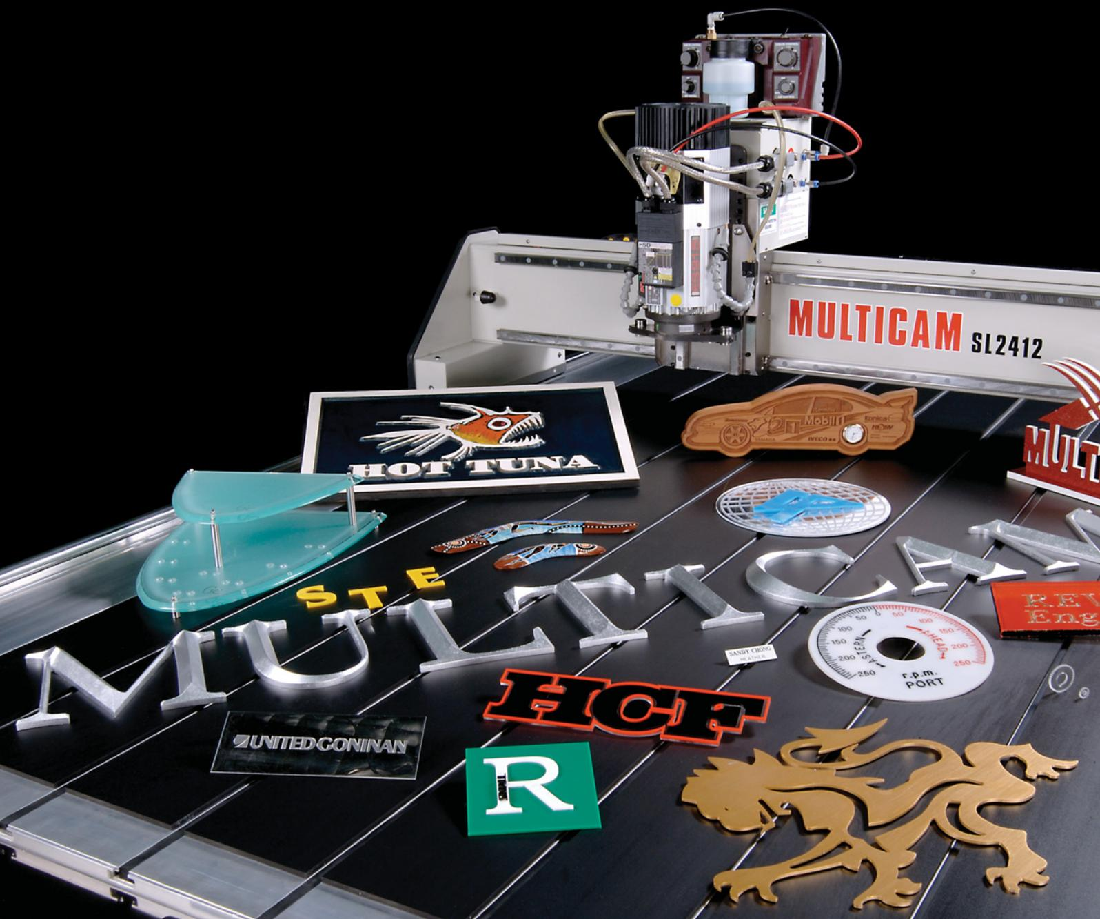
In the sign making industry you have to be versatile and fast. Two jobs are rarely alike. In the course of a single day you may be cutting aluminium, brass, plastic, timber, foam sheet or vinyl. The jobs may vary from a complex 3 Dimensional engraving, to cut out acrylic letters or making a vinyl face. The Australian Manufactured MULTICAM router handles them all with fast turn around time and minimal set up effort.
